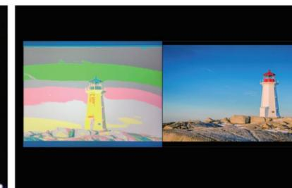
Special colors are used to indicate different levels of brightness in the image. Support ARRI, RED false color.
