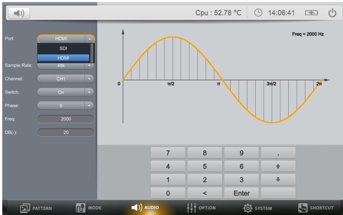
A comprehensive audio monitoring tool supports up to 16 channels embedded AES/EBU audio, with -60dB to 0dB range, And a 20Hz to 20000Hz frequency.
