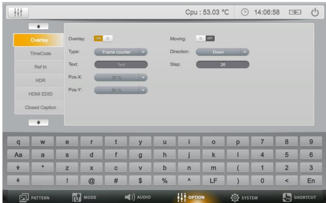
For solutions with various applications, the "Option" of device offers Overlay, image moving control and Ref In functions for users to analyze different signals and formats.
