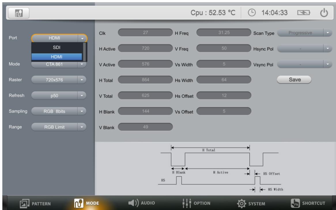
Mode interface supports switch the timing of output signal by using the keys or the mouse. And the related information of the signal output currently can be checked on the bottom of screen. (Timing sheet refers to Appendix 1)
