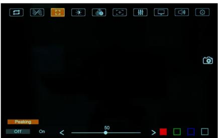
Use this item to activate or deactivate the peaking function. It is used to aid the camera operator in obtaining the sharpest possible picture.
