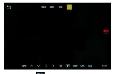
Tapping the "Camera" icon icon on the right edge to access the UI of camera control. Action in the UI of camera control are reflected to video camera in real time.
