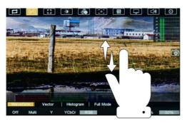
• Left swipe up or down: Adjusting the back light level.
