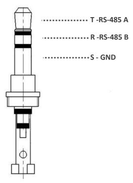
The Tally output pins on the receiver side are defined as follows.
